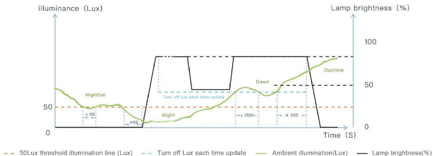
Ambient illumination and lamp brightness schematic diagram
