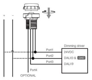
If the drive has no auxiliary power supply, an external power supply is required, It is recommended to use JL-710 built-in power socket
